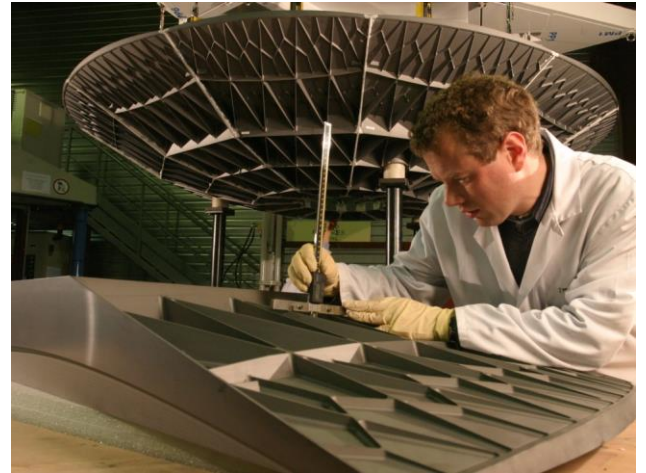
Fig.4. The HERSCHEL M1 is made of 12 SiC segments brazed together
