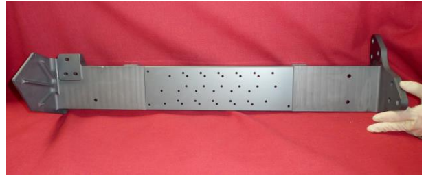
Fig. 9. The VNIR detector support (3.6 kg)
