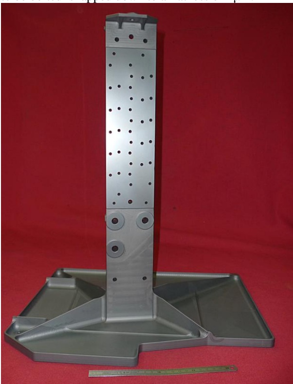
Fig. 8. The SWIR detector support (5.4 kg)
