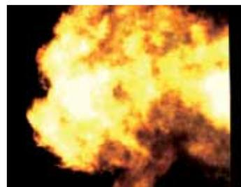
*A 22.8kA fault current is delivered to a circuit protected by a circuit breaker with a clearing time of 6 cycles. The resulting incident energy measured at 18" from the conductors was 8.14 cal/cm<sup>2</sup>, making Category 3 the minimum PPE required.*
