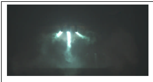
Fig. 3: Front view of arc development from vertical test 3ms into event.
