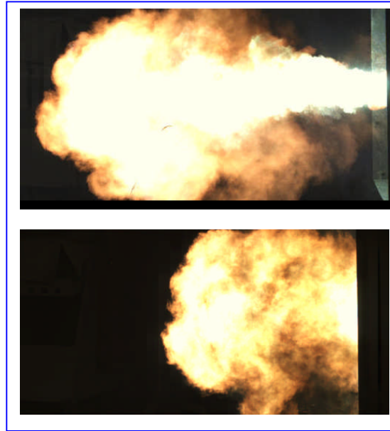
Fig. 7: Side view of plasma flow at 8 milliseconds into a 44kA 600V arcing event for horizontal electrodes. Electrode tips are flush with the front of the box (T) and recessed to 104mm from the back of the horizontal setup test box (B).
